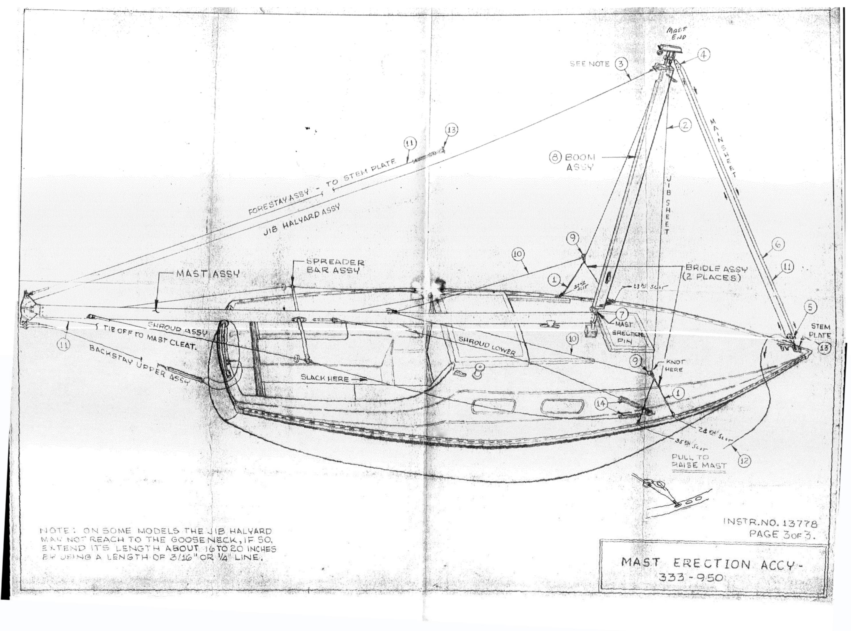
Shackle the two accessory mast erection bridles, #950, which are short lengths of wire with a thimble or eye in the center and one at each end, to the toe rail. One end attaches to the toe rail in the 23rd slot counting from the front. The other end attaches in the 32nd slot.
