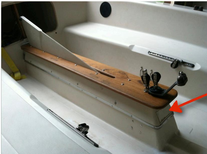
**Final note:** If I ever have to get back into the space below the cap, say to replace the blocks or something expensive like that, I would seriously consider cutting a window right here to get access without going through the rivet gauntlet again.
