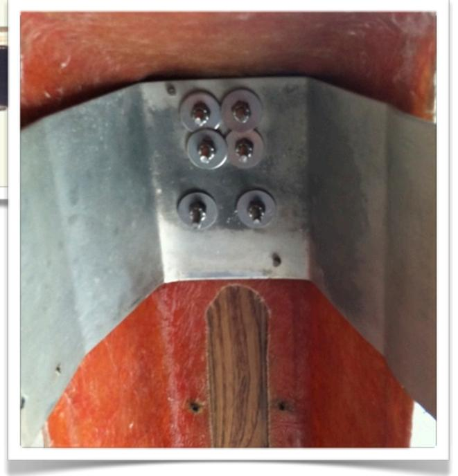
**Finishing up:** Replace the weather-stripping; reinstall the main-sheet block and swivel cleat/block with new stainless fasteners; re-rivet the cap to the base, or go big and use stainless screws instead of pop rivets. I used  $\frac{1}{8}$ " and  $\frac{3}{16}$ " aluminum rivets.
