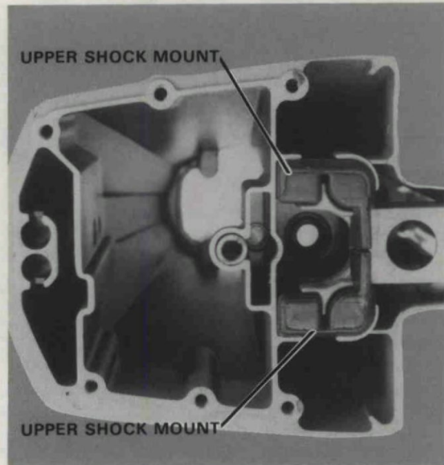
Figure 5. Upper Shock Mounts Installed.
